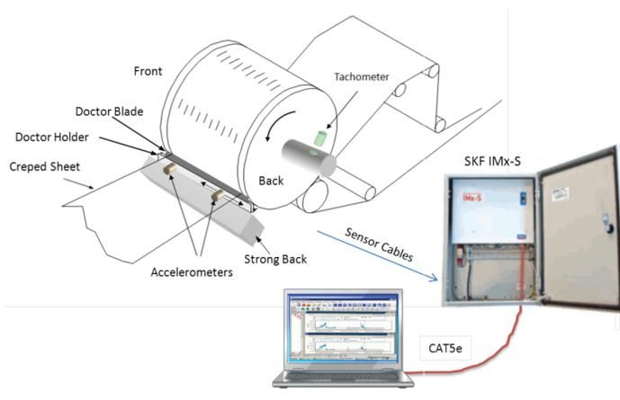
Figure 1 - Basic system diagram showing setup for crepe blade vibration monitoring system.
