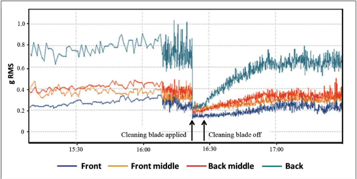
Figure 4 - Vibration intensity level (RMS) versus time showing the effect of loading the cleaning blade for a 15 minute time period. For this example data is shown for all four sensors.
