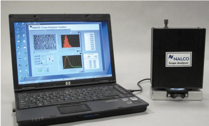
Figure 2 - NALCO system sensor head on right and lap top computer and software on left.
