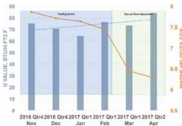
**Figure 2.** Overlaying heat transfer efficiency and flowrate to decide on cleaning needs.
