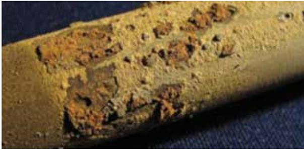
**Figure 4.** Photomicroscopy and deposit analysis results drive the decision to change cooling water treatment programme.
