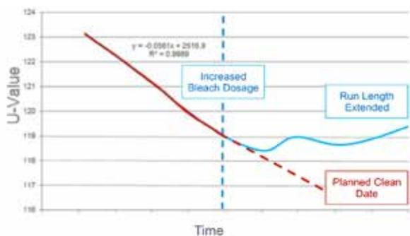
**Figure 1.** U-Value optimised with proactive monitoring of microbiological activity and chemical feed strategy.
