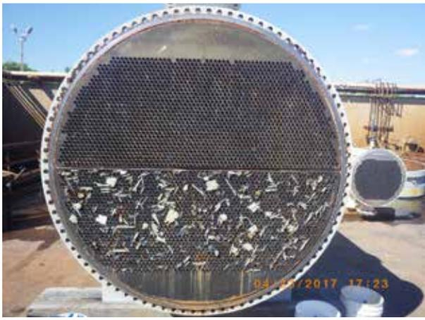
**Figure 3.** Debris in the inlet of the critical heat exchanger.
