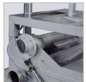
Automatic swivelling arm to prevent colour displacement
